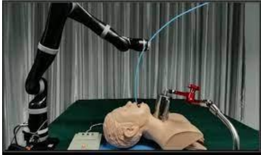
Fig 2.6: magnetically guided orotracheal intubation [19]
