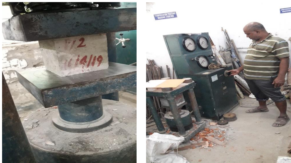
Fig. 5.10: Compressive strength test on concrete cube in laboratory.
