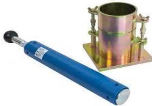
Fig. 5.3: Standard proctor mold and rammer diagram.
