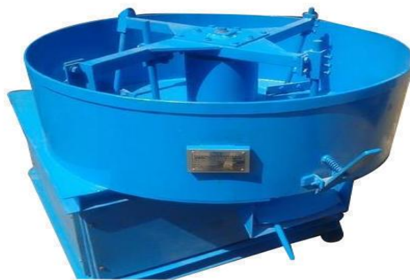
Fig. 4.6: Pan type concrete mixer machine.
