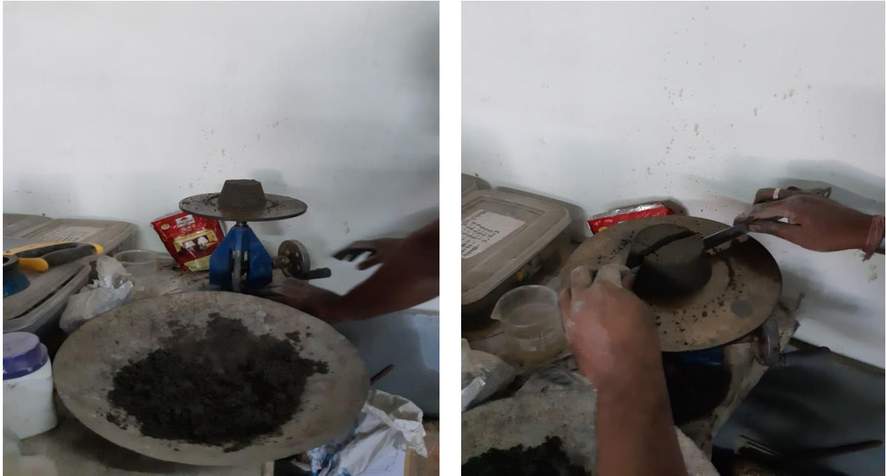
Fig:3.11 Mini flow table test procedure and measurement of flow diameter.
