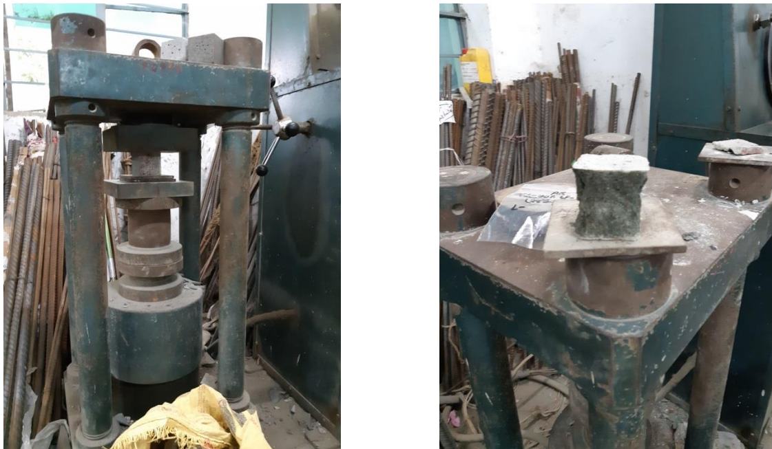
Fig-3.14: Compressive strength test set up and failure pattern of sample after compression.
