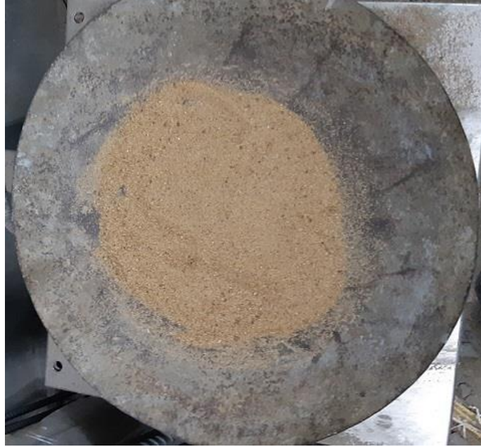
Fig:3.3 Sand conforming to grading zone-II
