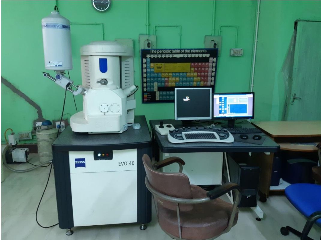
Fig-3.17: Scanning Electron Microscope instrument (courtesy GSI SEM-EDX lab kolkata).
