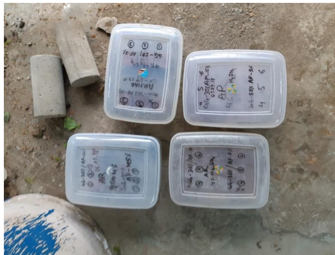
Fig-3.15: Samples stored in 4% H 2 SO 4 and MgSO 4 solution in laboratory.
