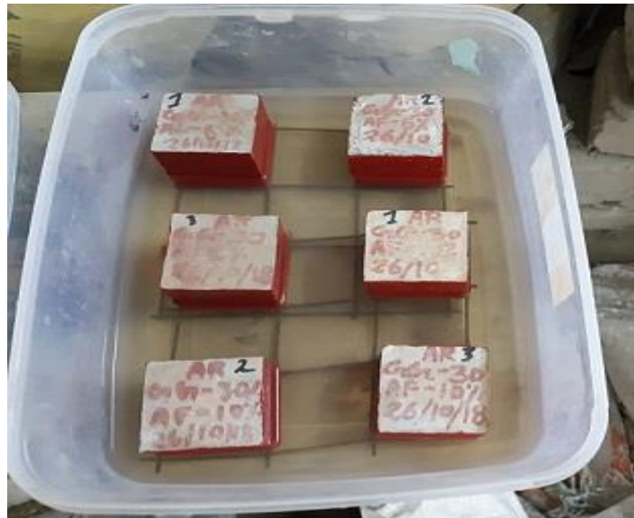
Fig-3.13: Test set up for sorptivity.
