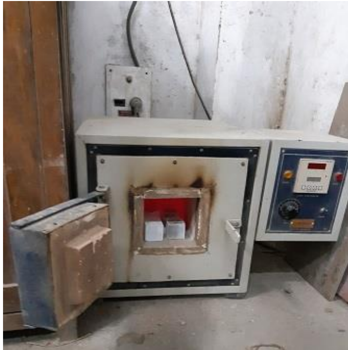
Fig-3.16: Samples exposed to high temperature at furnace .
