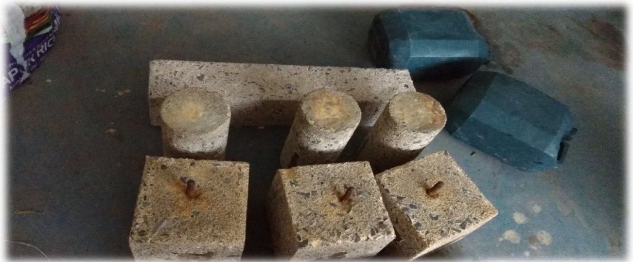
Fig6.3 Specimens after removal from H 2 SO 4 solution
