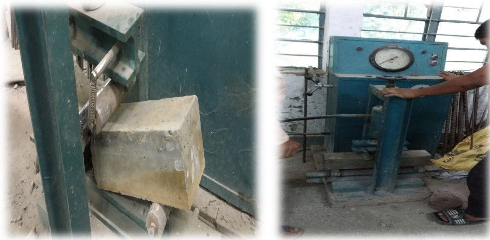
Fig.5.14 Flexural strength Test central point loading in laboratory
