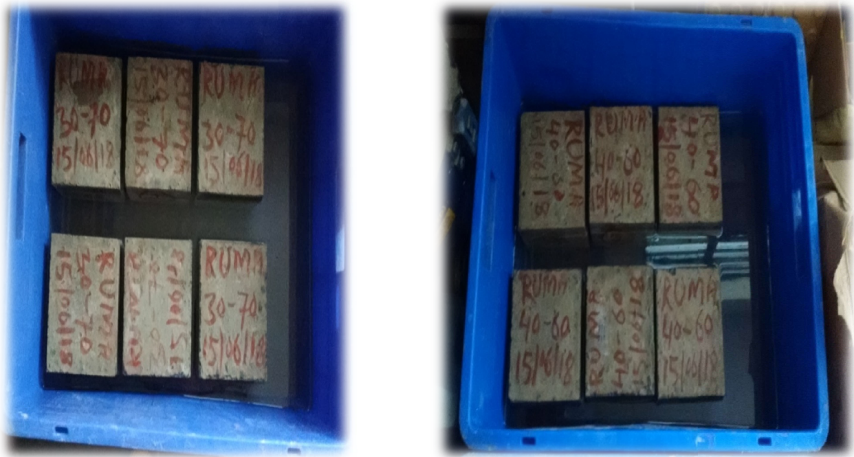
Fig 6.1 specimen immersed in MgSO 4 solution
