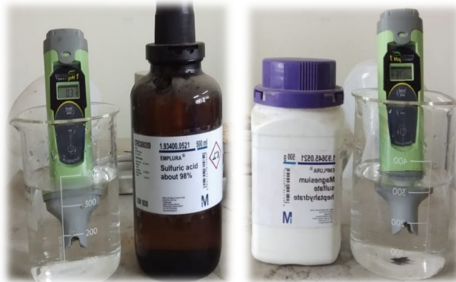
Fig.5.10 Acidity test of sulphuric acid and magnesium sulphate solution
