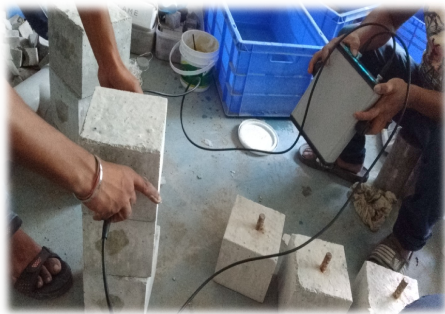
Fig.5.16 Ultrasonic pulse velocity Test in laboratory
