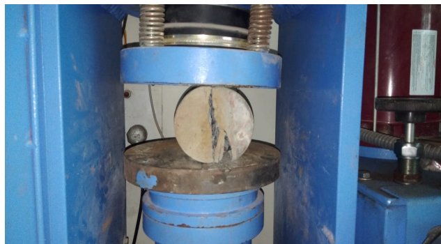
Fig.3.26 Failure of Cylinder
