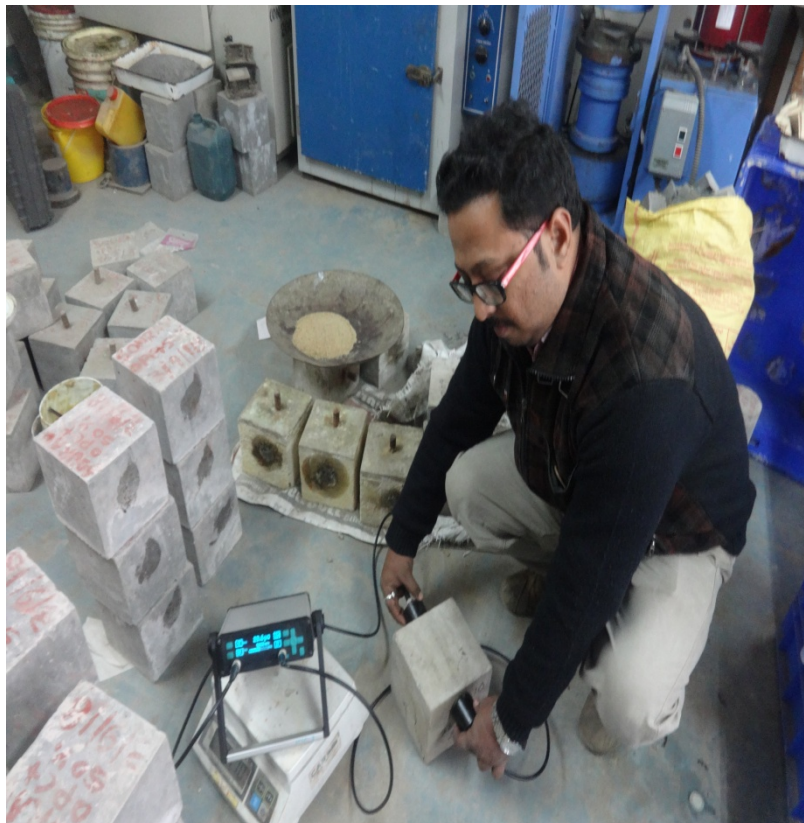
Fig.3.32 Ultrasonic pulse velocity test in laboratory
