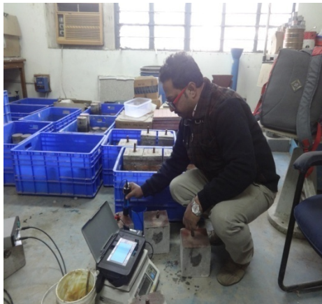
Fig.3.35 Half-cell potential testing in lab
