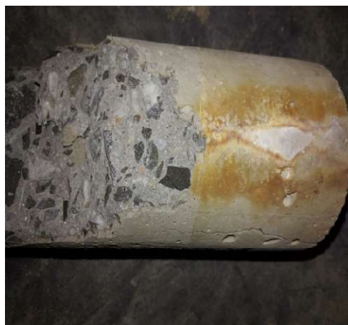
3.27 Outer and Inner surface of a Cylinder after 4 months acid exposure
