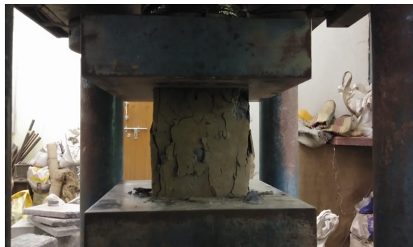
Fig.3.25 Failure of cube in compression
