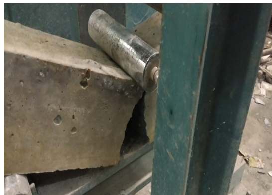
Fig.3.29 Failure of Beam
