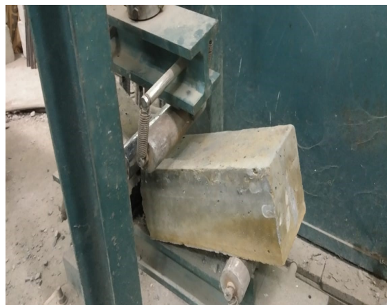
Fig.3.30 Failure of Beam
