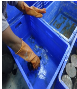
Fig.3.10 Mixing of Acid with water for curing of the samples
