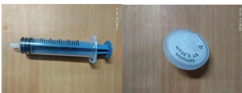
Figure 6: syringe filter (Sartorius NY 0.2 \mu L )
