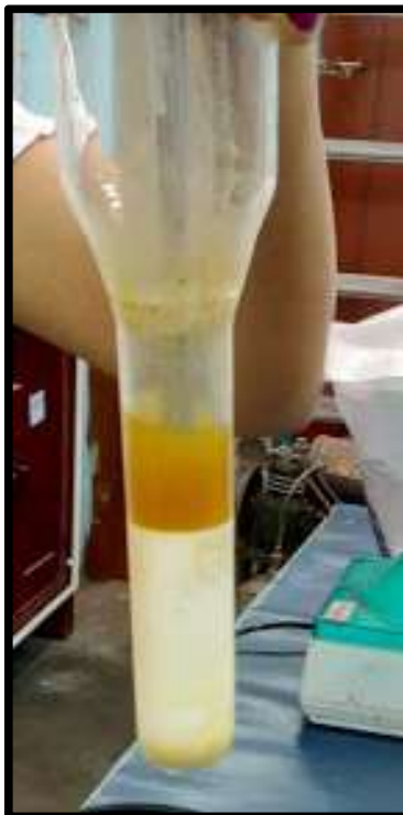
Figure 11: Homogenisation of depigmented biomass using Chloroform-Methanol mixture
