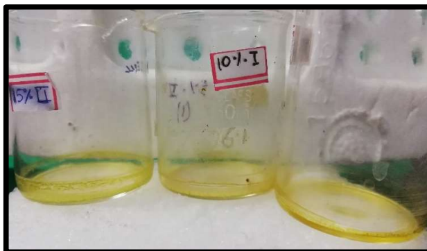
Figure 13: Supernatant containing algal lipid and extraction solvent post drying
