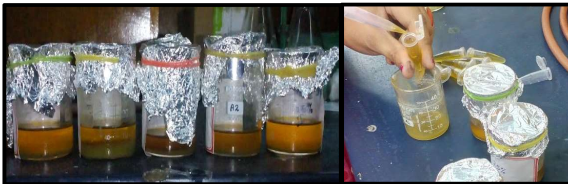
Figure 12: Homogenised mixture being prepped for centrifugation
