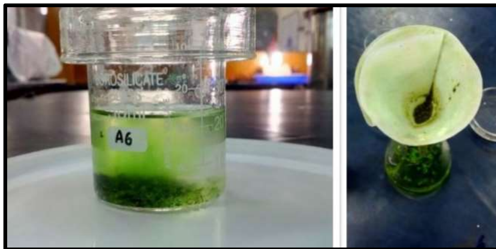
Figure 10: Depigmentation of algal biomass using Acetone-NaOH mixture followed by filtering out of the depigmented biomass for lipid extraction
