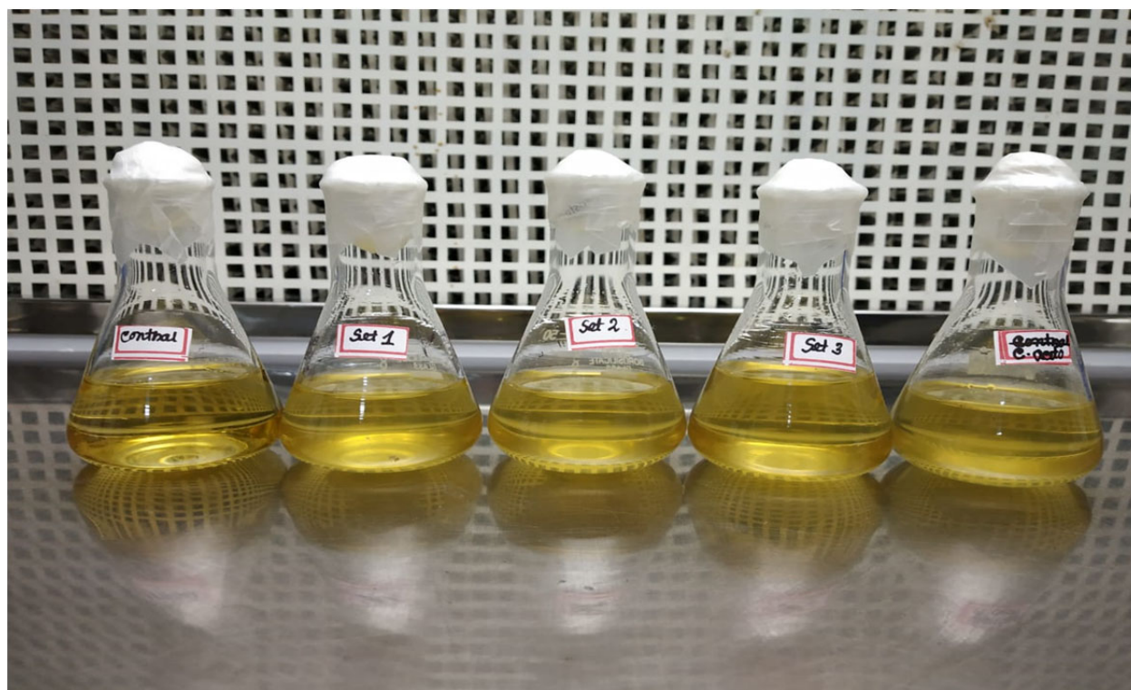
Figure 35: Different sets inoculated in RCM containing effluent of acidogenic consortium and Clostridium acetobutylicum inoculate.
