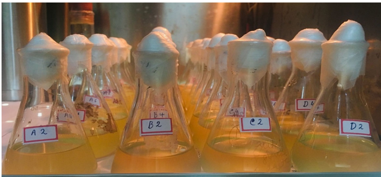
Figure 10: Batch study with varying concentration of glucose and hydrolysate as substrate
