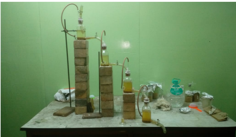
Fig 9: Exp. Set-up of PFR (Plug Flow Reactor)
