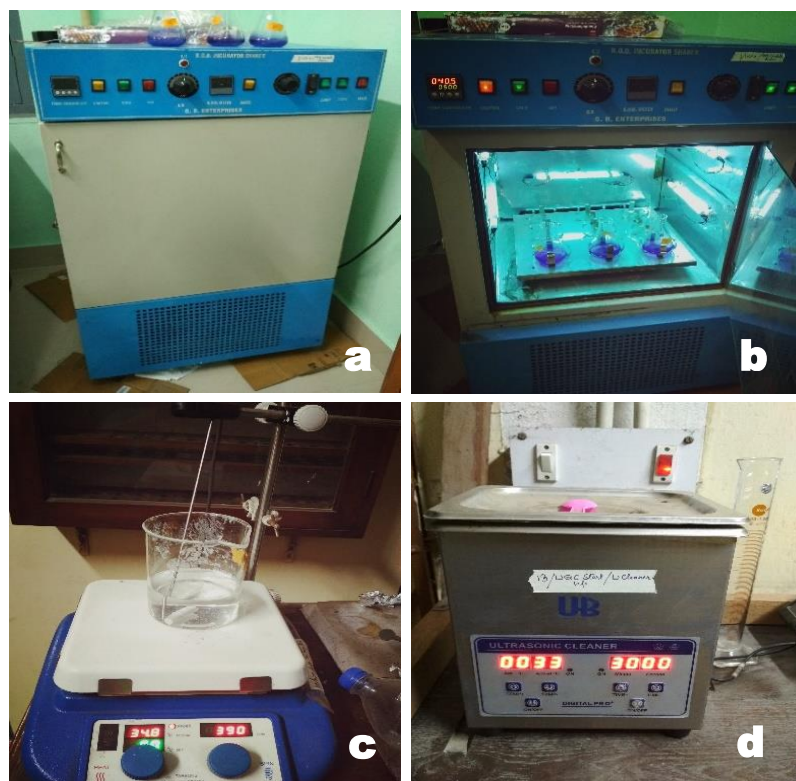
Figure 3.4 Image of instruments (a) (b) Incubator shaker, (c) Hot plate stirrer and (d) Sonicator
