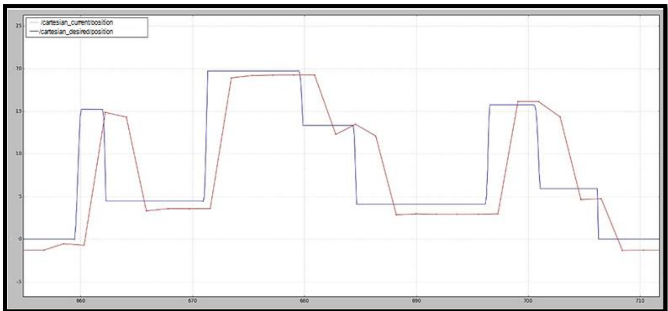
Figure 6.2 Position of joystick and UR5 end effector in Y axis.
