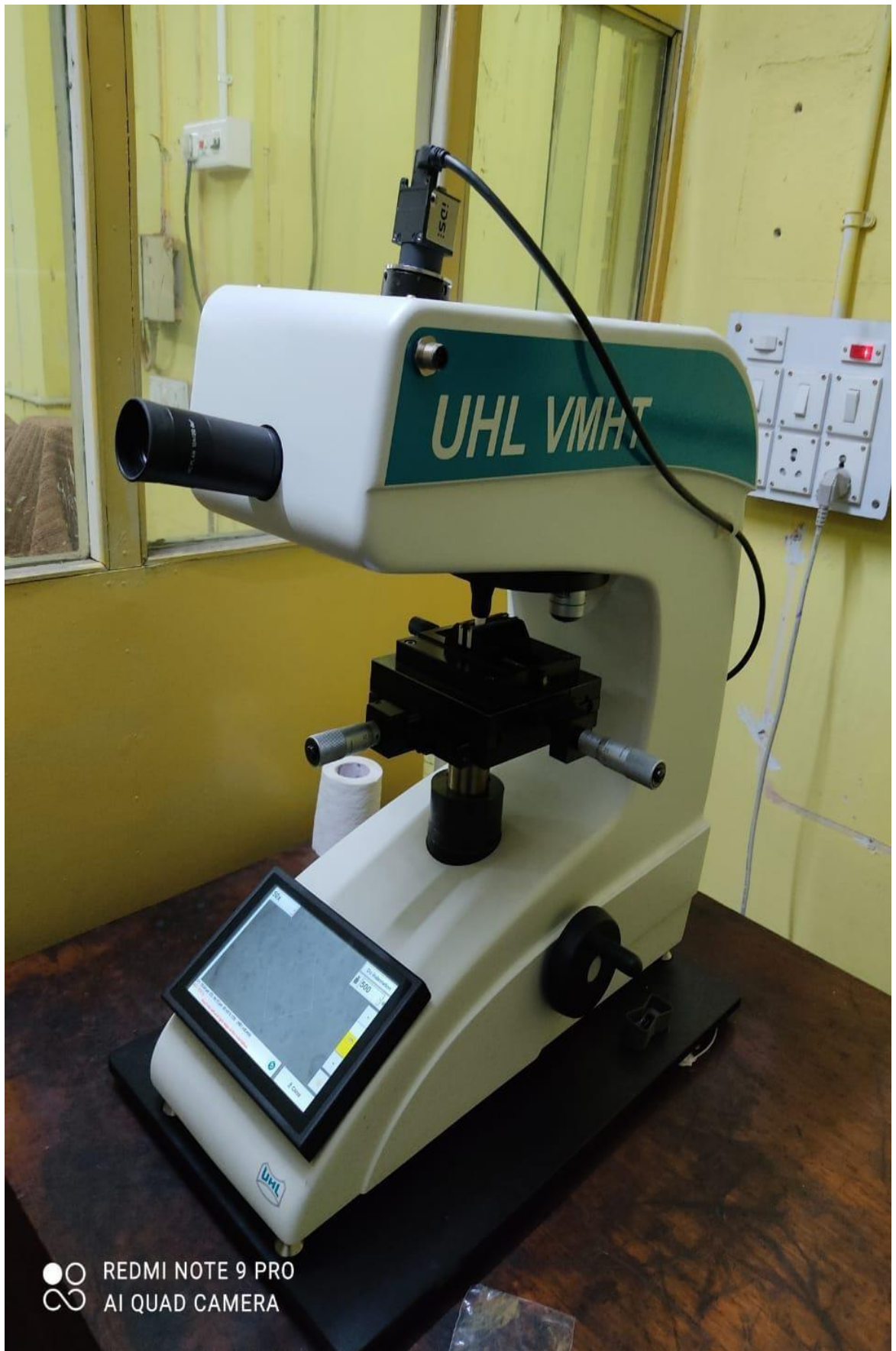
FIG-3.13-Pellet Is Being Placed Under Indenter And Micro-Hardness Is Being Tested
