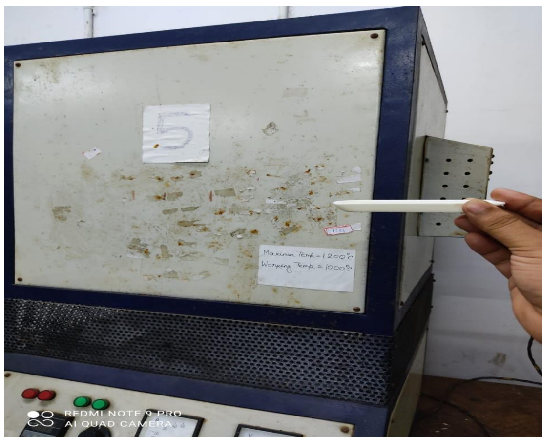
FIG-3.5.-GEL IS PLACED IN A BOAT AND PLACED IN A FURNACE FOR CALCINATION
