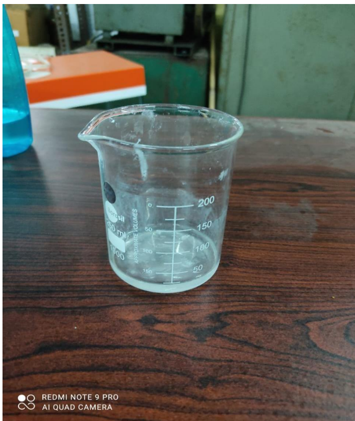
FIG-3.2-AFTER WEIGHING,RAW MATERIALS WERE MIXED TOGETHER WITH 10ml. DISTILLED WATER
