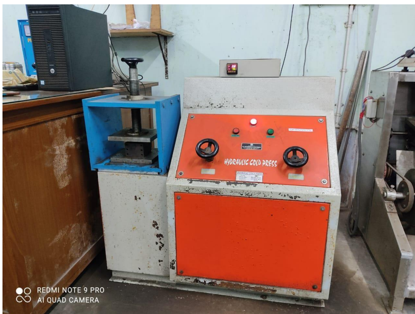
FIG-3.7-PVA MIXED CALCINED POWDER IS BEING PRESSED IN HYDRAULIC COLD PRESS
