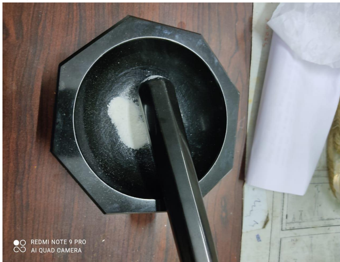
FIG-3.6-CALCINED POWDER IS GROUND IN AGATE MORTAR
