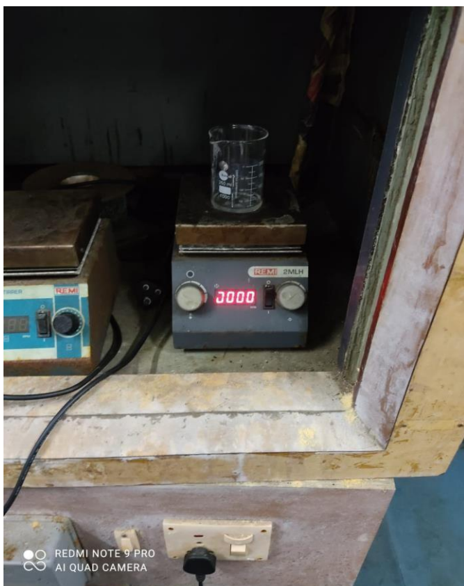
FIG-3.3- AFTER COMBINING TOGETHER, THEY WERE HEATED AT 80°C FOR 3 TO 4 HOURS TO FORM GEL
