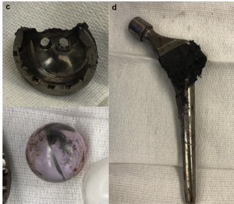
Figure 5.1 Fracture polyethylene liner and femoral head, acetabular wear because of erosion
