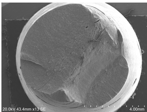
4.15(a) SEM fracture morphology of specimen of 60 MPa mean stress (b) fracture morphology of the same showing micro-voids
