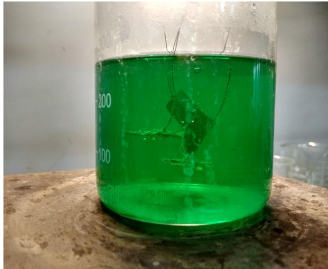
Fig 15. Electroless bath with the copper substrate placed over the heating plate
