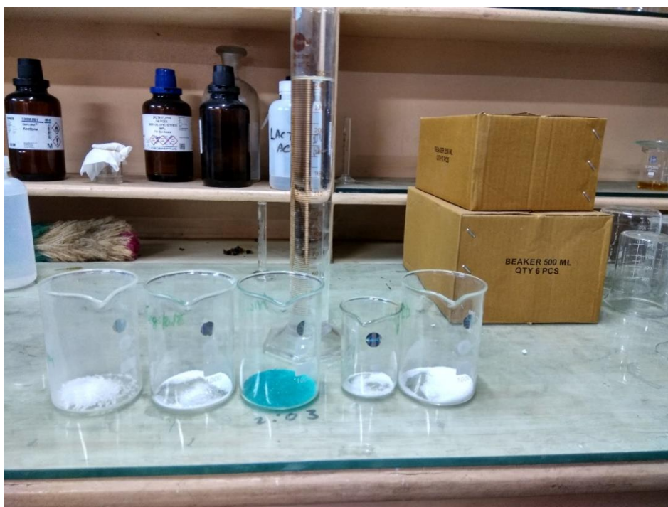
Fig. 4. Electroless bath preparation having a bath volume of 250 mL
