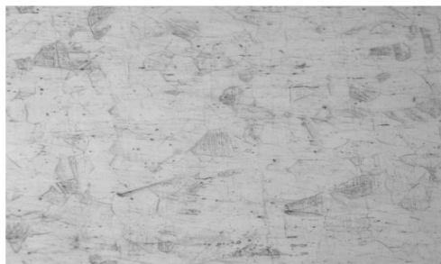
Figure 3.21 Metallographic view of sample number: BASE METAL 304L
