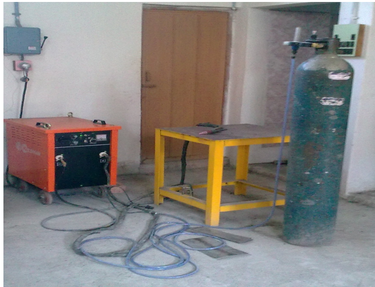
Figure 2.1 Tungsten inert gas welding machine used in the work
