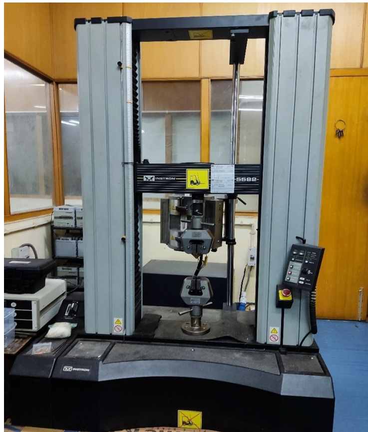
Figure 2.3 Photographic view of Instron universal testing machine
