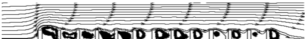
Fig. 4.13: Velocity streamline when inlet velocity is 30 cm/sec
