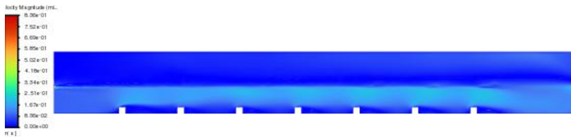
Fig. 4.14: Velocity contour when inlet velocity is 10 cm/sec
