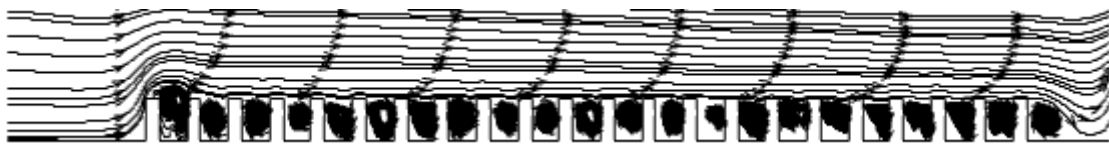
Fig. 4.4: Streamline when inlet velocity is 10 cm/sec
