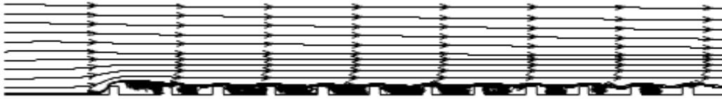
Fig. 5.4: Velocity streamline for intermediate-type roughness ( p/k=5 )
