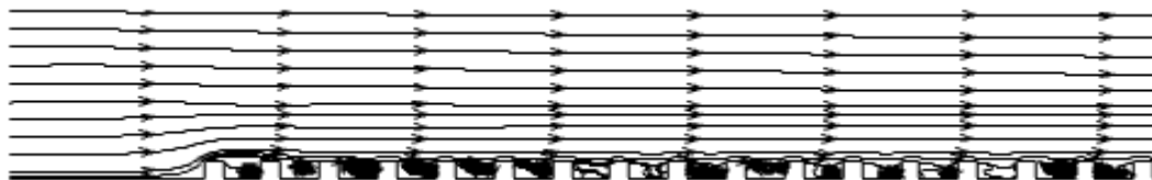
Fig. 5.2: Velocity streamline for d-type roughness ( p/k=3 )
