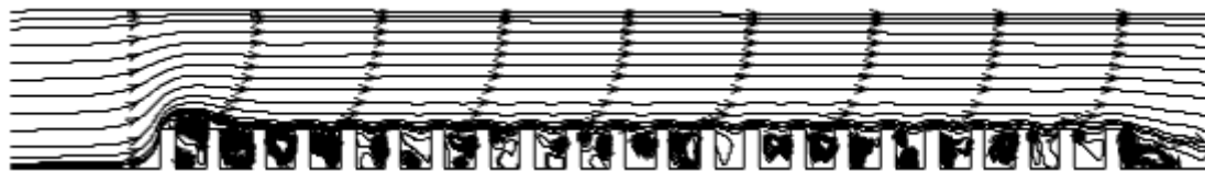
Fig. 4.5: Streamline when inlet velocity is 20 cm/sec
