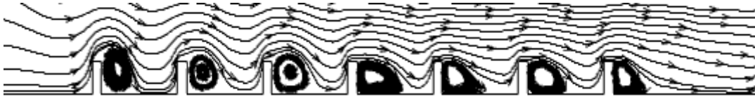
Fig. 4.17: Velocity streamline when inlet velocity is 10 cm/sec
