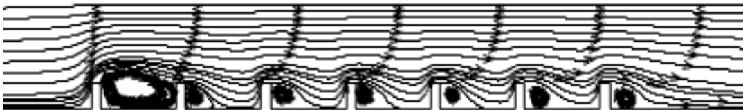
Fig. 4.18: Velocity streamline when inlet velocity is 20 cm/sec
