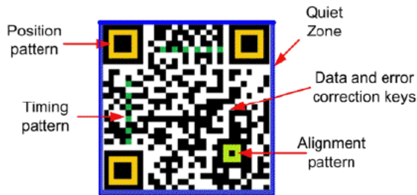
Fig 14: Internal Structure of a QR image
