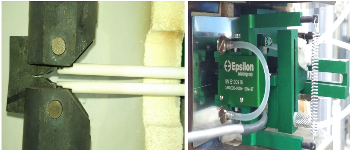
Fig.3.6: Half CT specimen during the room temperature J-test is in progress.
