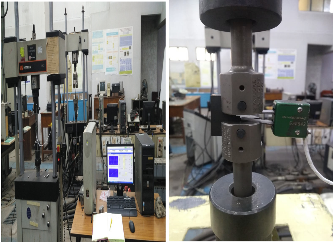
Fig. 3.5: Set-up used for pre-cracking of the specimens.
