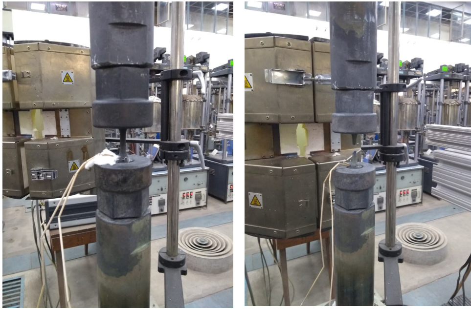
Fig. 3.4: Set up for high temperature tensile test.
