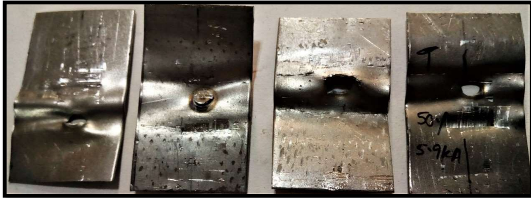
Fig 4.3 After peel test at 5.9 KA
