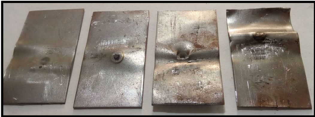
Fig 4.2 After peel test at 5.0 KA
