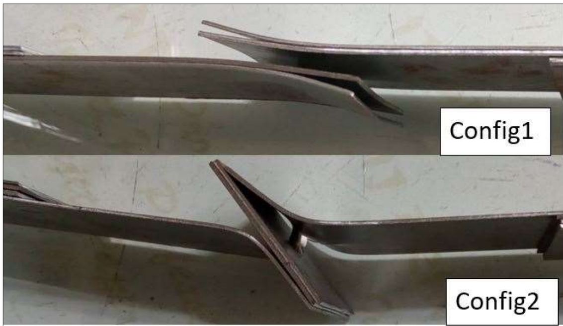
Fig 4.11 Config1 and Config 2 after failure
