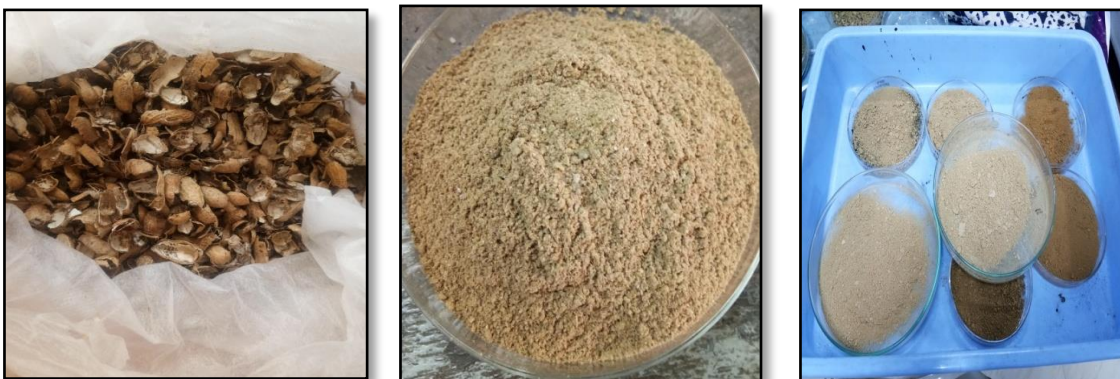
Figure 2.1-(Peanut shell waste) (Groundnut after milling) (Peanut After Pretreatment)
