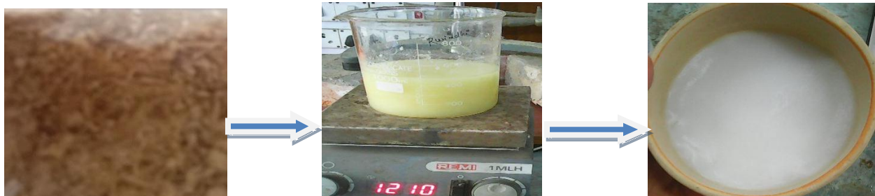
Fig 9: Nanocellulose extraction from Raw sugarcane bagasse fibers
