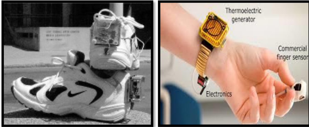
Fig 1.24 The shoe-powered RF tag system By piezoelectric energy harvesting Fig 1.25 Human based Energy Harvesting using body heat
