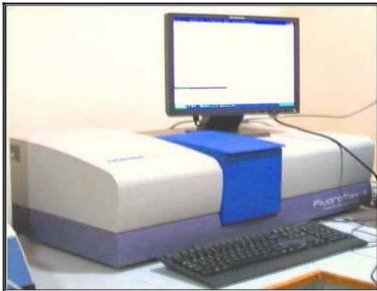
Figure. 4.21 Experimental set up of SHIMADZU RF-5301PC Spectrofluorometer.
