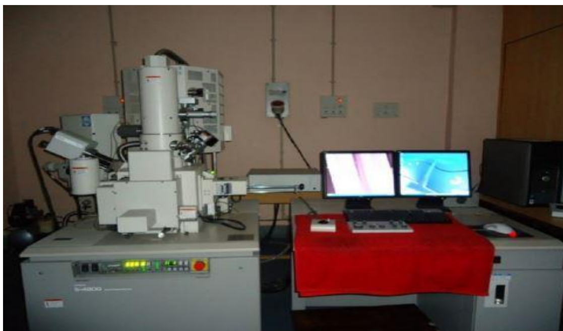
Figure 4.12: Hitachi S4800 FESEM with EDX attachment
