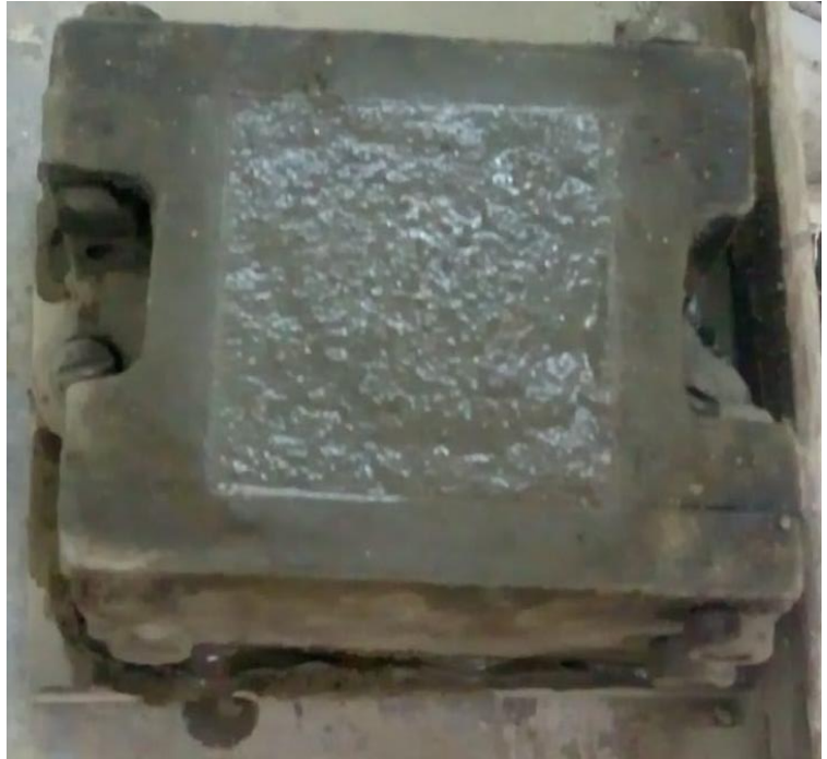
Fig.: 18 Prepared GO Cement Mortar
