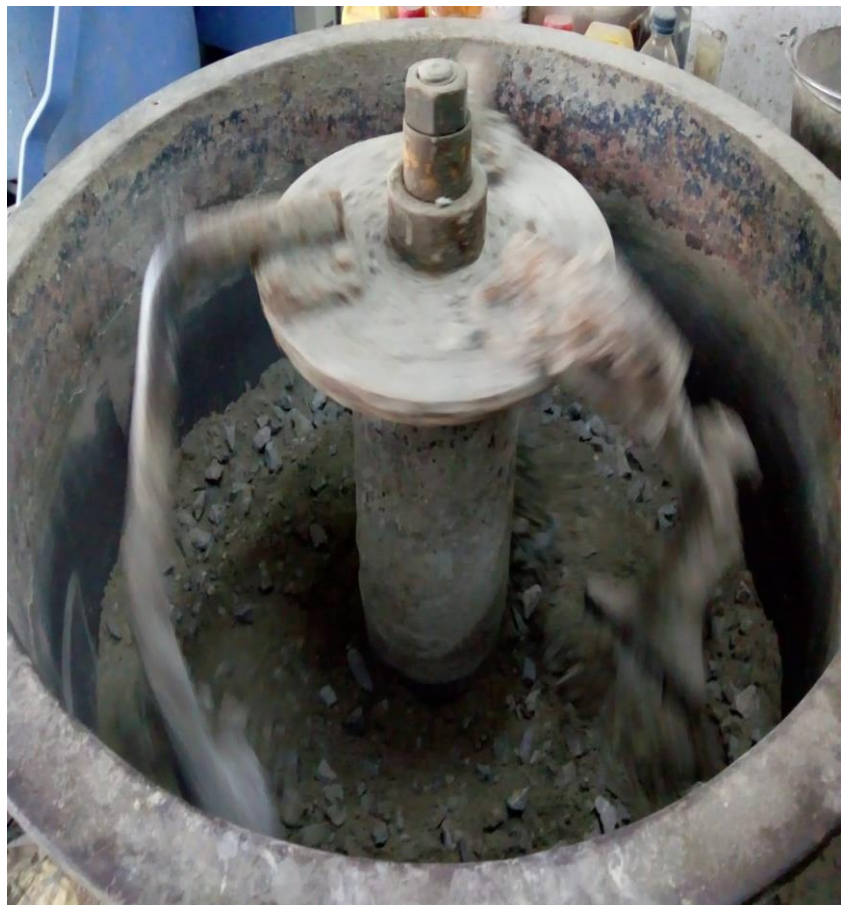
Fig.30: Mixing of sand, cement, plastic dust & aggregate
