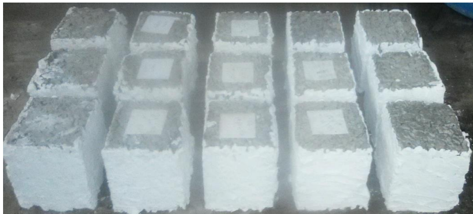
Figure 3. 3 Specimens for permeability test covered with plaster of Paris
