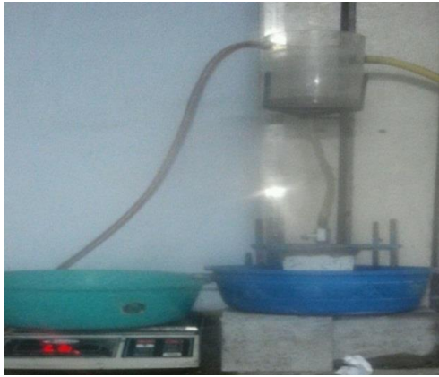
Figure 3. 4 Permeability tests set up
