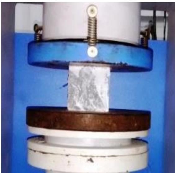
Fig 3.4 Compressive Strength Test by Compression Testing Machine
