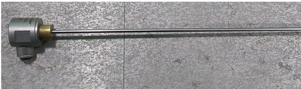
Fig 4.2a: Stringer attached with load cell at the top
