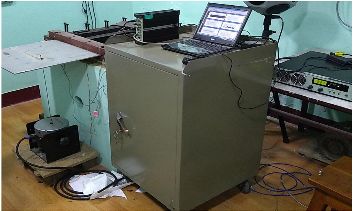
Fig 4.2d: Complete setup of shaker test
