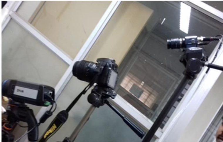
Figure 1: Camera Setup showing the cameras corresponding to the thermal, visible and near-infrared spectrum (left to right)
