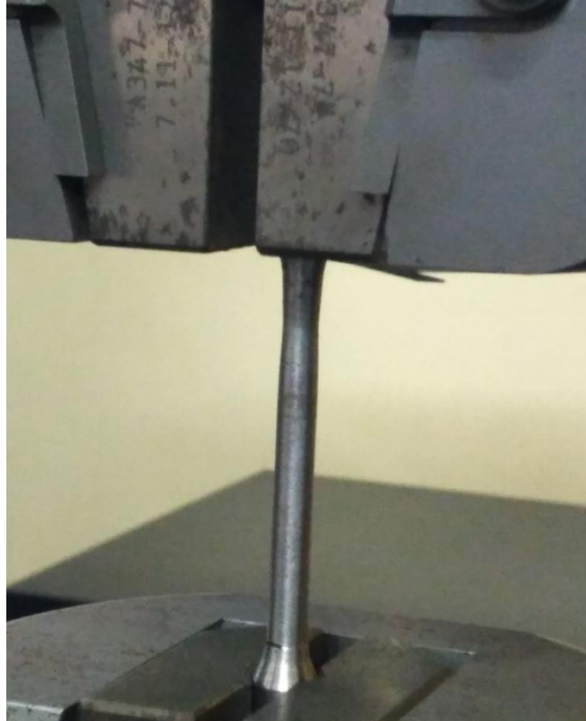
Fig 3.3(c): Tension Test of Mild Steel Specimen
