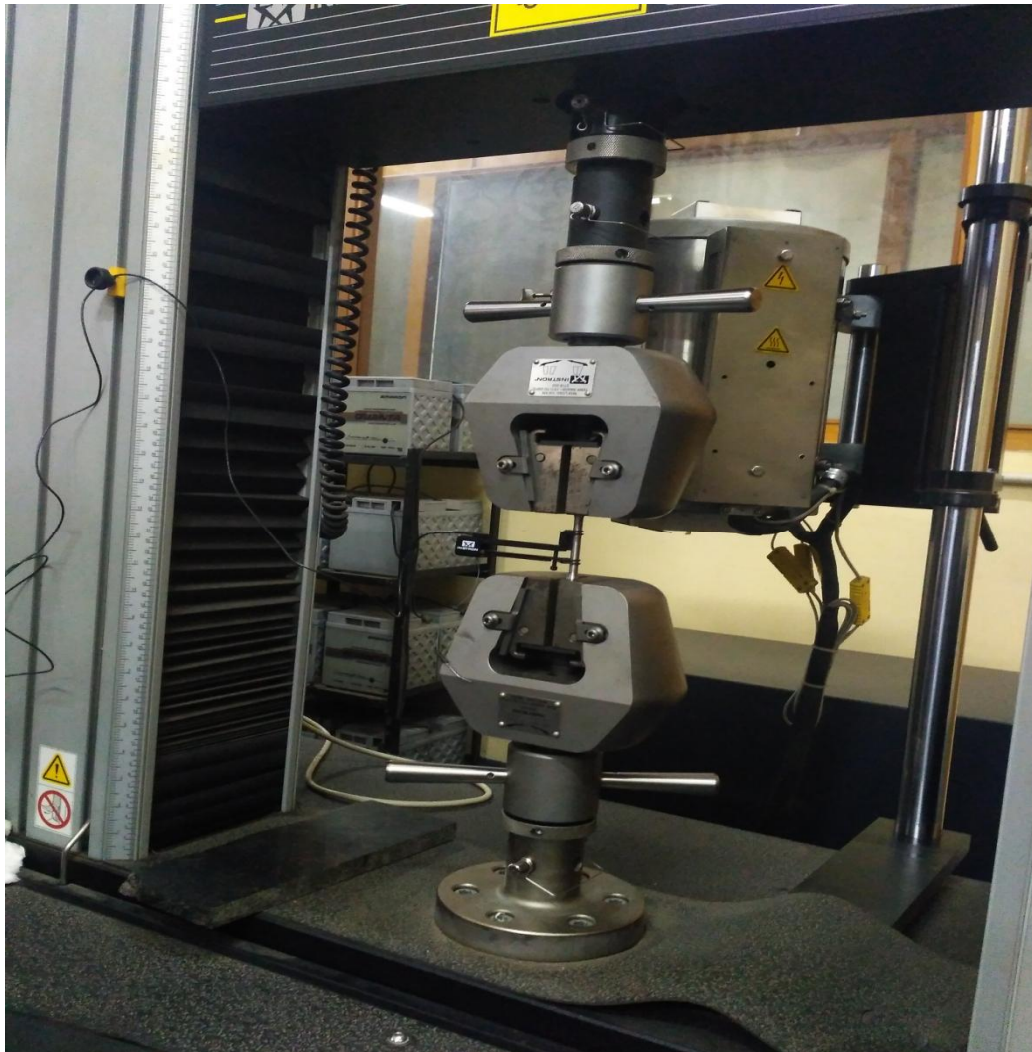
Fig 3.3(b): Tension Test of Mild Steel Specimen
