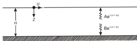
Figure 2.2: Linear elastic soil deposit of thickness H underlain by rigid bedrock
