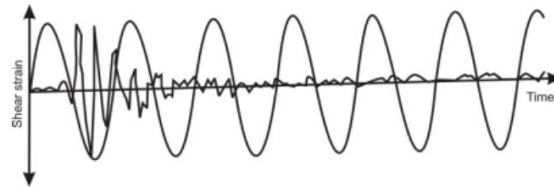
Figure 2.5: Two shear strain time histories with identical peak shear strains. For the transient motion of an actual earthquake, the effective shear strain is usually taken as 65% of the peak strain
