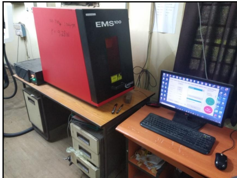
Fig. 3.1: Laser cutting setup (ELECTROX EMS 100)
