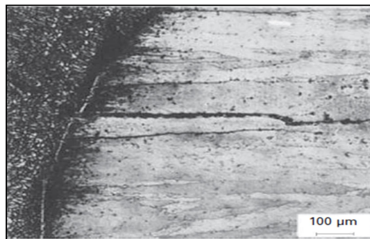
Fig.2.14 HAZ liquiation crack in laser welded sample
