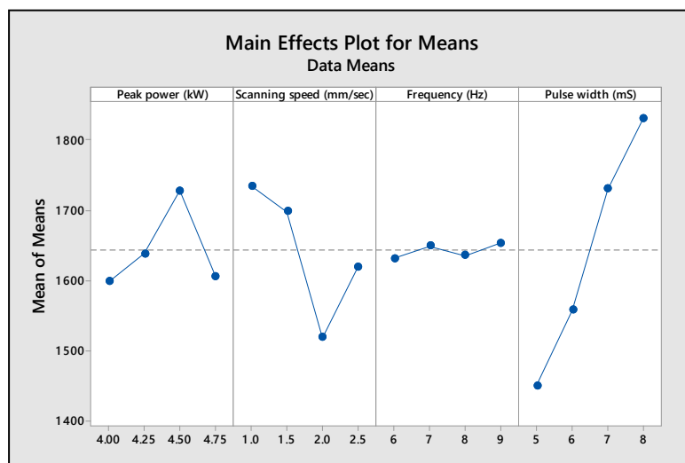
Fig. 3.34: main effects plot for welding width
