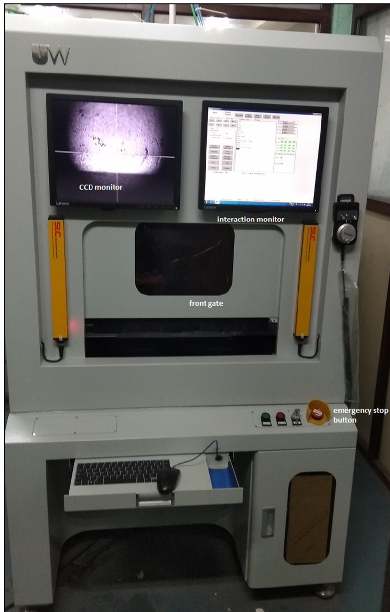
Fig 3.2 Laser welding machine
