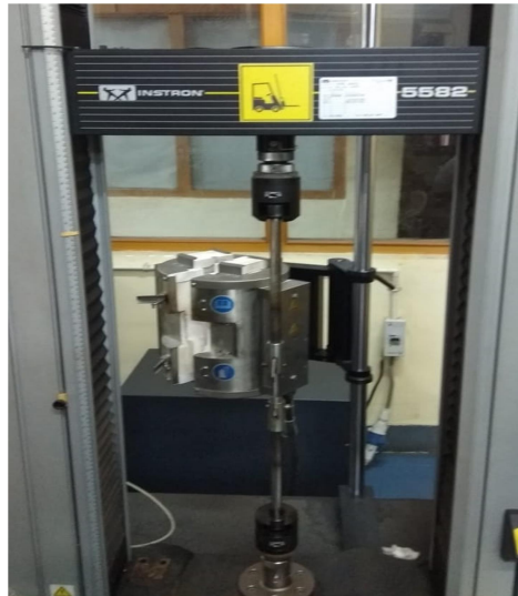
Fig. 3.8 Pictorial view of universal testing machine
