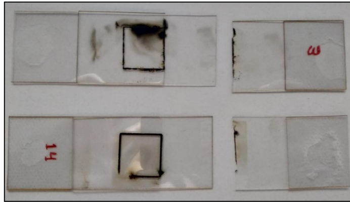
Figure 3.8 Photograph of the samples having the highest ultimate load (experiment no 3) and lowest ultimate load (experiment 14)
