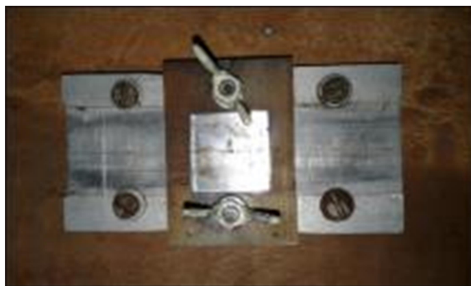
Figure 2.7 Clamping device used for welding
