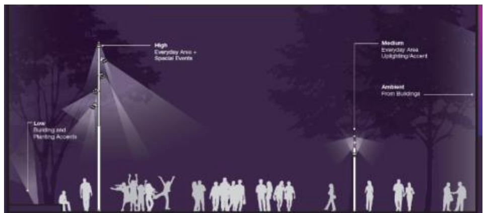
Figure 76 Image & section of street lighting on the key routes
