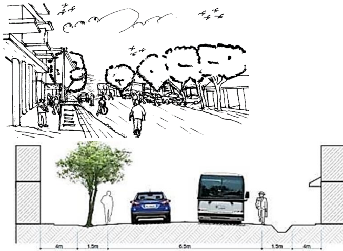
Fig.3.19 Mbalizi road – (Collector)
