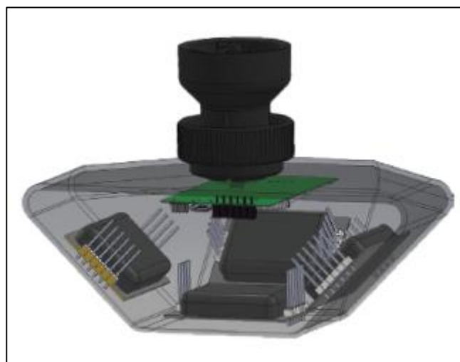
Fig 3.11: Internal details of the Sensor Module
