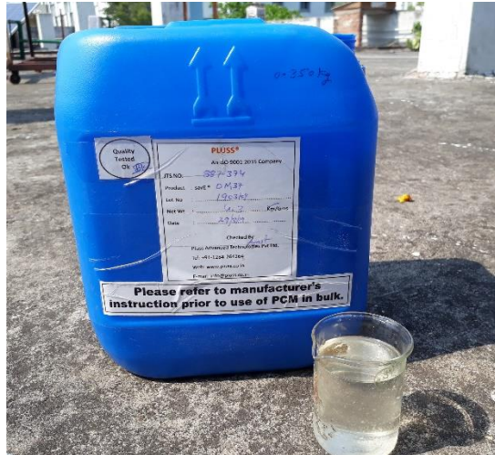
Figure 5.1 & 5.2 Sample of PCM in solid & liquid state [pic courtesy PLUSSTech]
