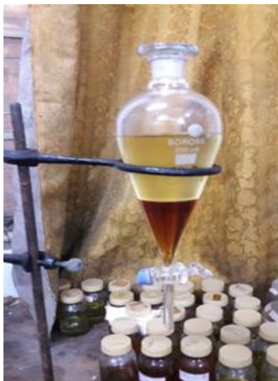
Fig 5.7: Separation of biodiesel and glycerin
