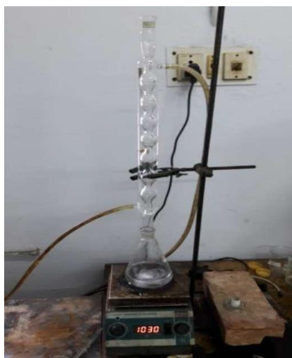
Fig 5.5: Methanol and KOH Mixing
