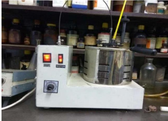
Fig 7.3: Apparatus for Flash and Fire point measurement
