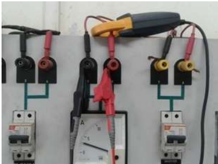
Figure 5.5 Connection for DC Measurement
