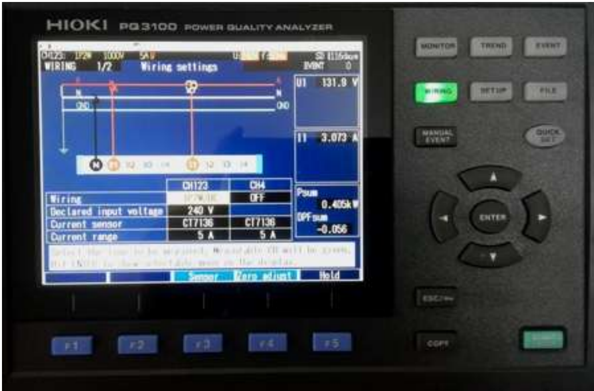
Figure 5.7a Wiring (HIOKI PQ3100)
