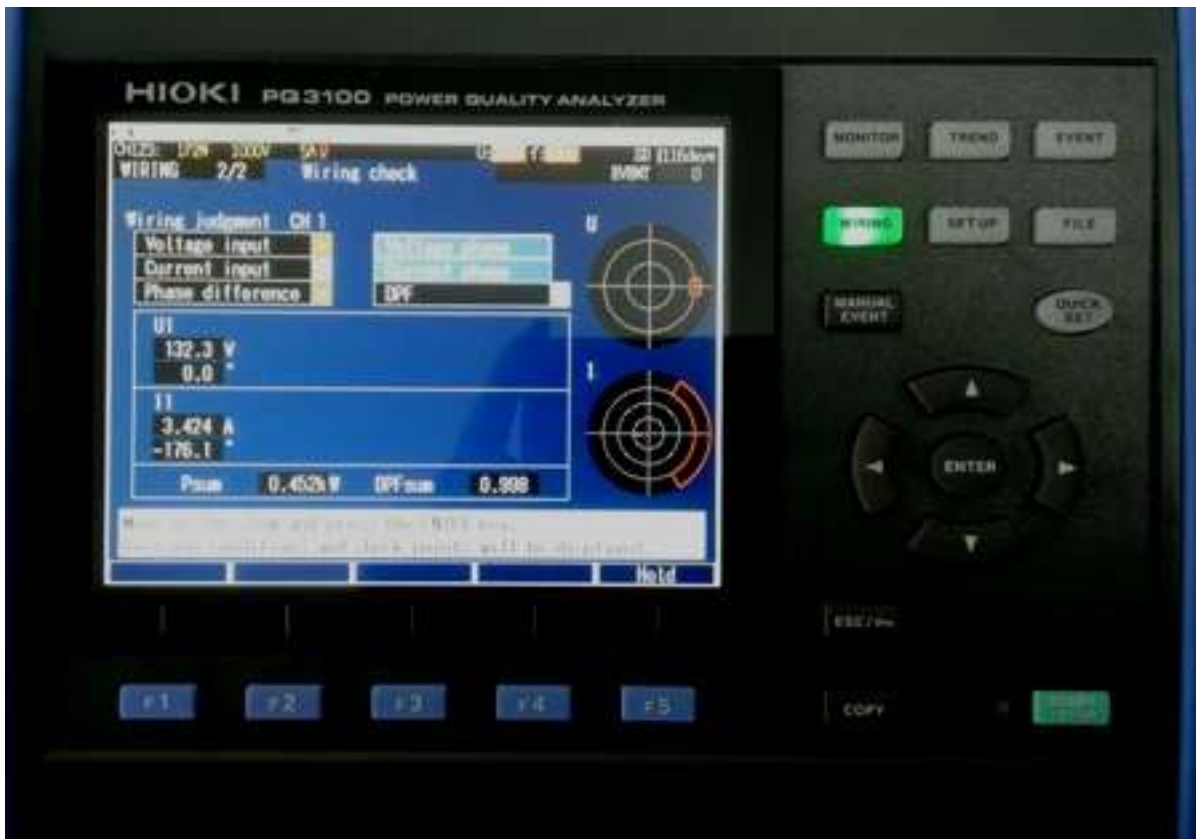
Figure 5.7b Wiring (HIOKI PQ3100)
