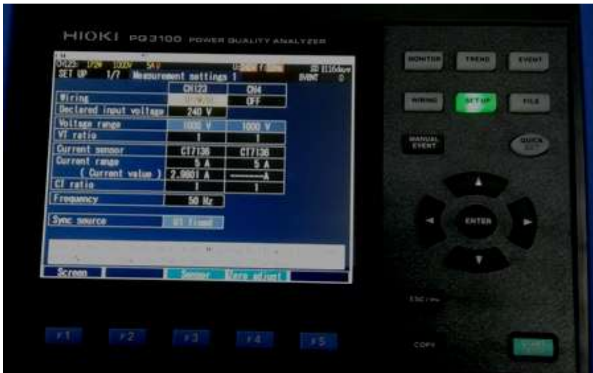
Figure 5.6 Setup (HIOKI PQ3100)
