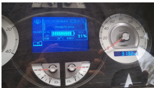
Figure 2.1: view of the display behind the steering wheel of the electric bus
