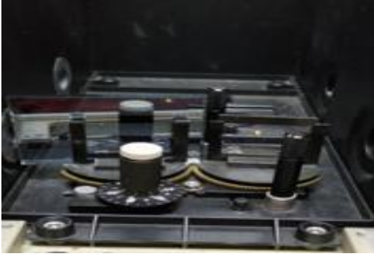
Fig 4.3 Setup for measuring spectral transmittance
