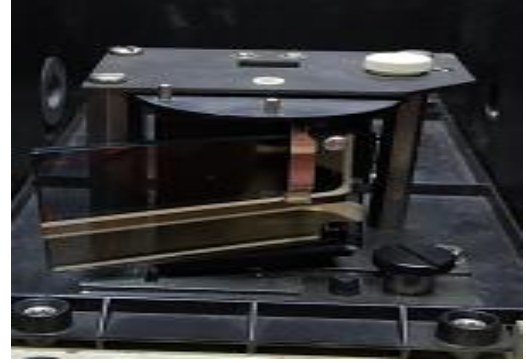
Fig 4.4 Setup for measuring spectral reflectance
