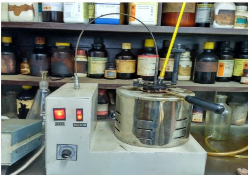
Fig.2.3 Flash point measurement set up
