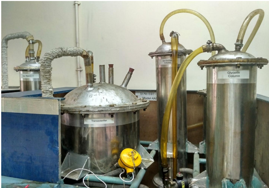
Fig-5.3 : Glycerol column (extreme right), Transesterifier(center), Auxiliary column (extreme left)
