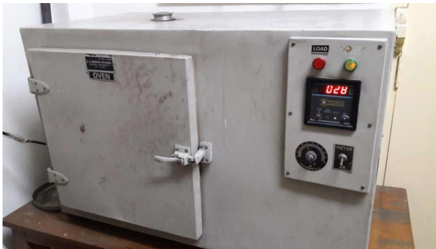
Fig-4.8 : Air oven for remove moisture from biodiesel
