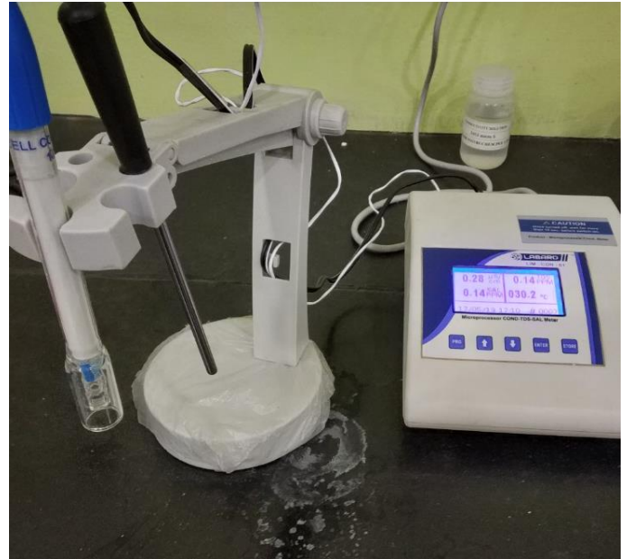
Figure 5. 6 Conductivity and TDS Meter at Plant
