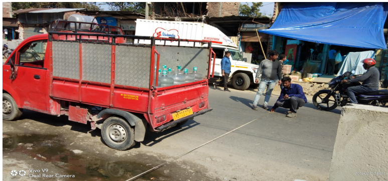
Photograph 4.1: Measurement of carriageway width in market place
