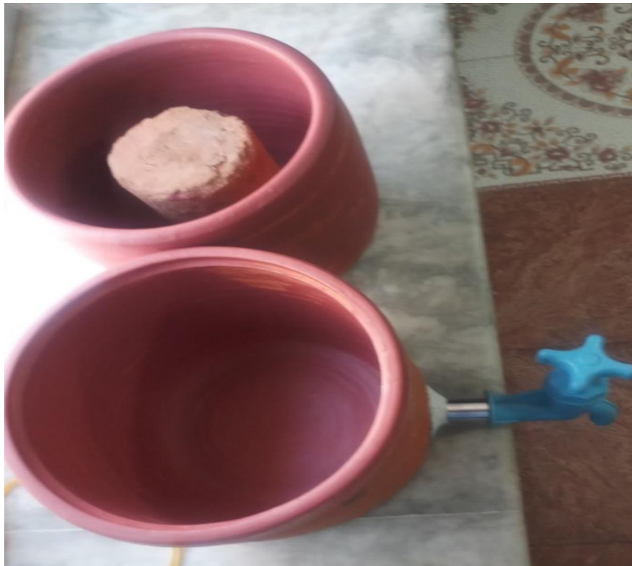
Filter is ready for working- Figure-5.4.3
