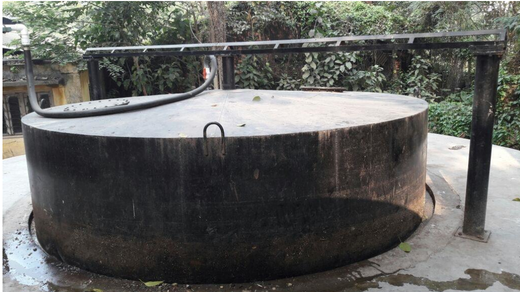
Mesophilic digester with floating drum gas holder
