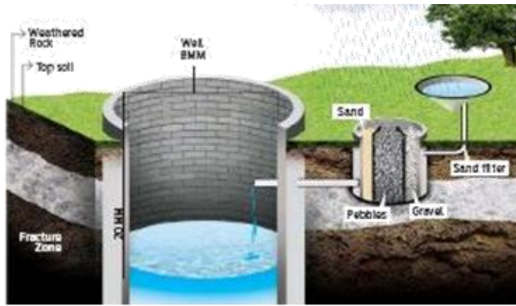
Induced recharge structure, Dharmapuri district, Tamil Nadu
